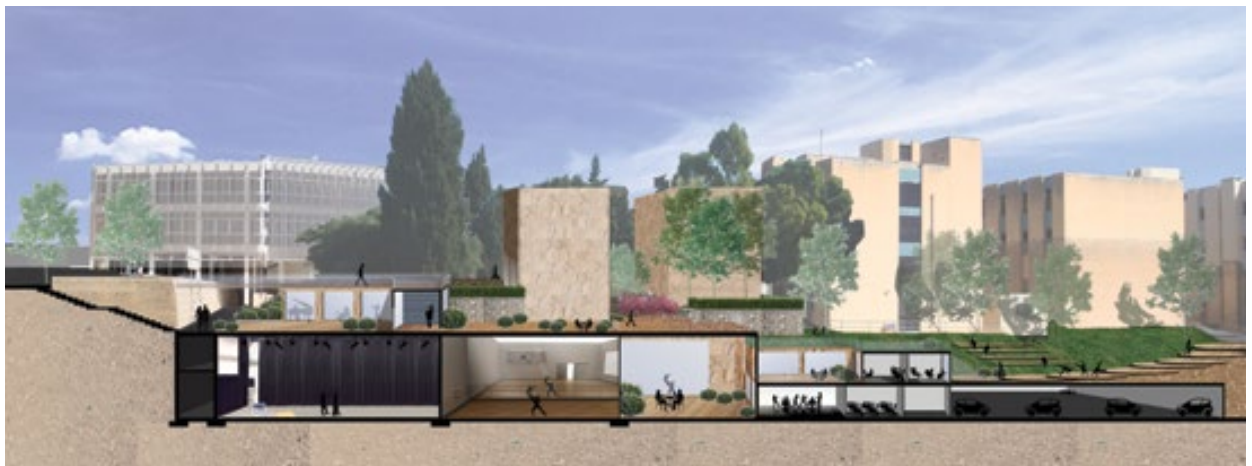
A cross-section view of the new terrace proposed beneath Atriju Vassalli, housing a car park, lecture rooms and spaces for the School of Performing Arts.
